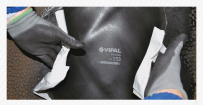
The patch should be applied with the beads in original position, not opened.
