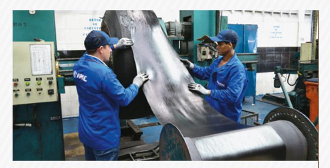
After preheating the tread compound, apply the OTR binding, using the same procedure as the tread compound, which can be applied directly to the tyre/tire or saved in spools.
