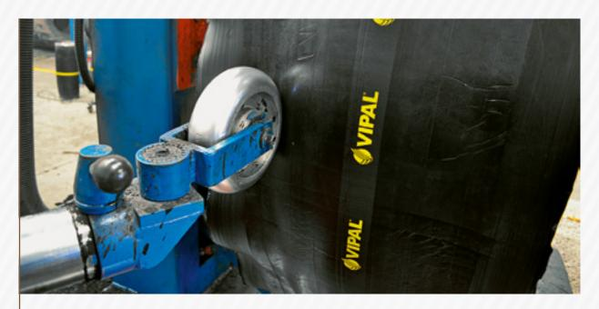
Activate the pneumatic tread pans on the rolling machine so that they work from the hump to the edges, eliminating air from beneath the Camelback.
