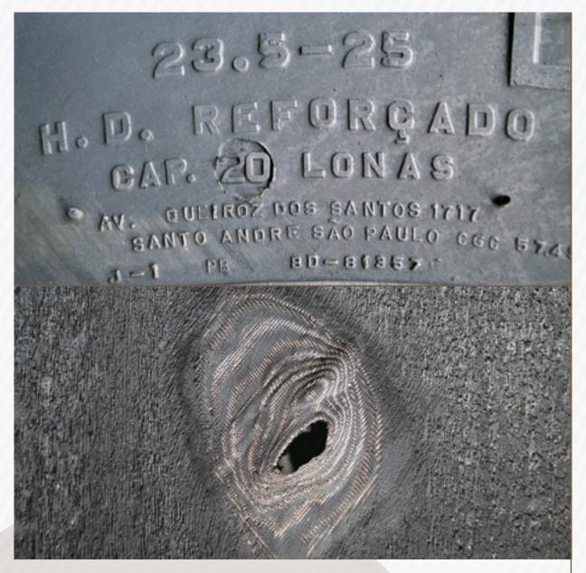
Damages should be measured on the first outer ply, disregarding the protective plies.
