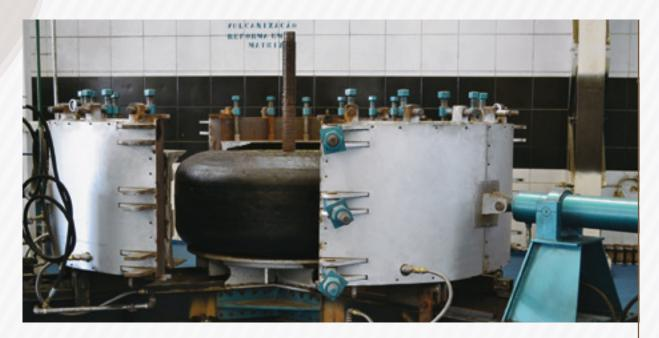
Place the tyre/tire centered in the machine, without leaving gaps between sectors, in order to prevent staggered formation.
