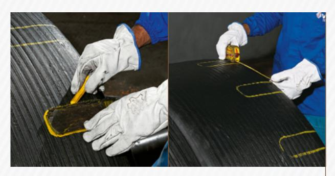
Tyre/Tire with autoclave vulcanization design: After covering, mark the chosen design through a template.
