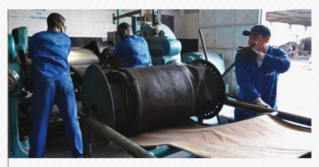
Continue to prepare the rubber to coat the tyres/tires by heating the compound by passing it back through the cylinder and withdrawing the thickness from 7 mm to 10 mm, storing them on a mat or spool.
