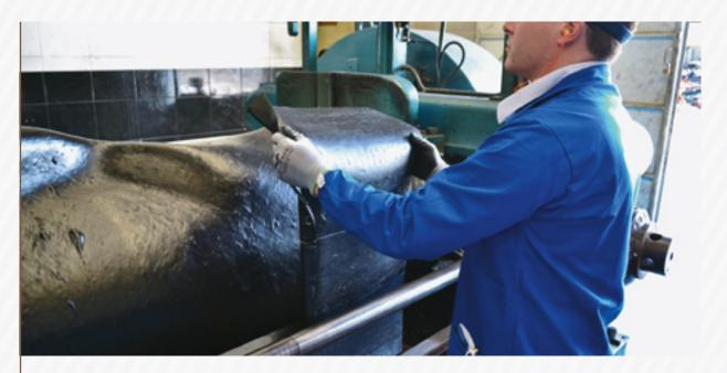
Cut the compound into pieces to feed the cylinder.
