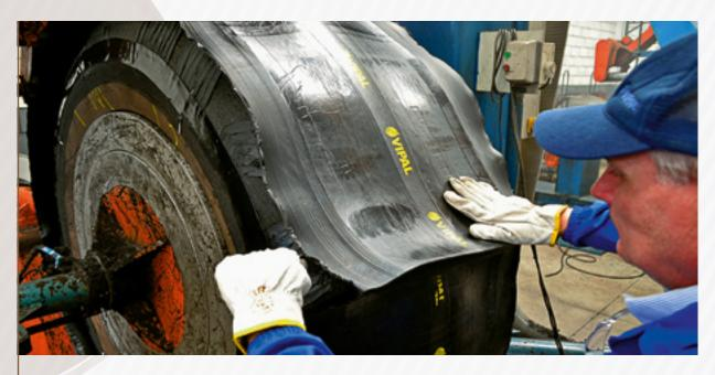
For perfect adhesion of the Camelback patch, its length should be 10 to 15 mm longer than the tyre's/tire's perimeter. With the aid of a metal ruler, position the ends, hit it with a rubber hammer to increase the patch pressure, and fix it with a proper instrument.
