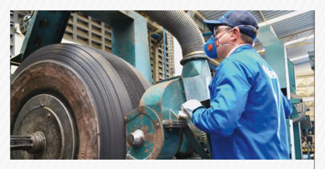
Buff the tyre/tire always from the hump toward the sides, ensuring that at the end the sub-tread offers a sufficient rubber base for adhesion and protection of the nylon plies and/or steel belts.
