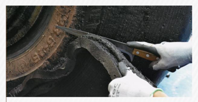
After rolling it, remove excess material.
