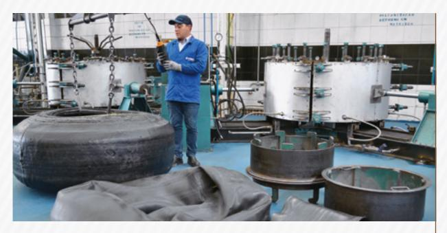
Assemble the tyre/tire with air bag, protector and wheel. Before placing the tyre/tire in the matrix, spread a demolding agent if necessary.
