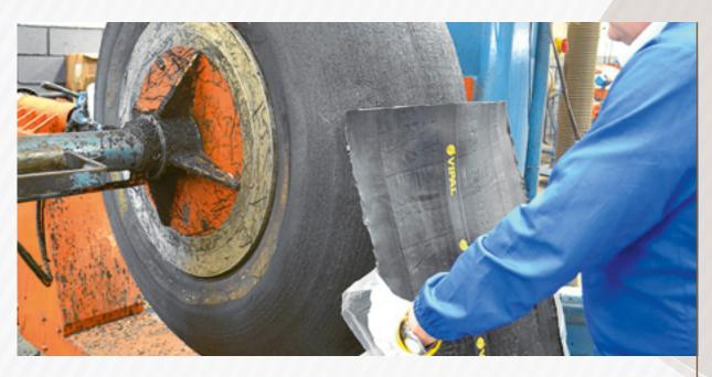
Position the tyre/tire in the machine and inflate it to 15 to 20 psi. Remove the piece of plastic from the Camelback, avoiding contact with the cushion. Center it and fix one of the tips on the tyre/tire.
