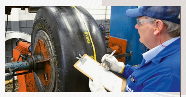
Measure the perimeter to check the measurements.
