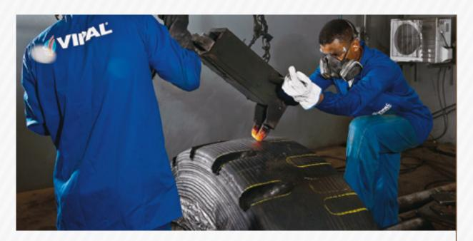
Place the tyre/tire in a trench or filleting stand. Proceed with the design filleting according to the chosen model, depth, and base.
