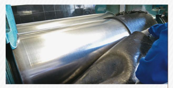
Start the compound homogenization passing it through the cylinder, performing 5 (five) to 6 (six) cuts. Warm-up time is approximately 5 to 10 minutes.
