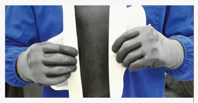
Remove the protective film from the patch from the hump to the edges, leaving room to hold the repair and prevent base contamination.
