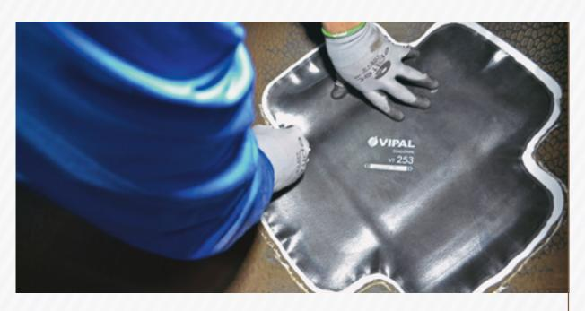
Keep the tyre/tire in normal position, without opening the beads. Position the template or patch at the center of the damage and mark the outline with chalk.
