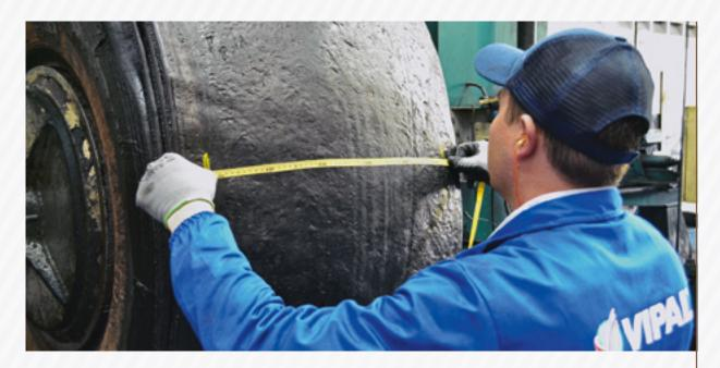
With the tyre/tire covered, set and demarcate the tyre/tire tread width.
