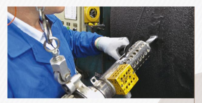
With an extruder heated to  $75^{\circ}\text{C} \pm 5^{\circ}\text{C}$ , fill the skives with Cushion gum, leaving no more than 1 to 2 mm excess above the tyre/tire level.
