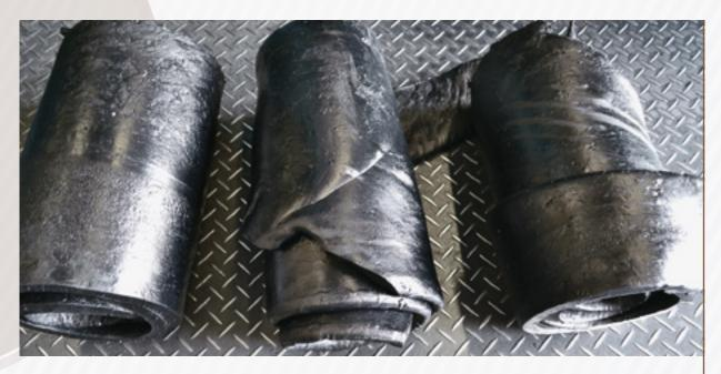
After compound homogenization, remove coils of 15 to 20 kg and store them on pallets so that there is a space between the rollers, facilitating ventilation.
