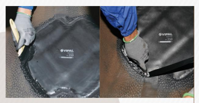
When vulcanizing occurs in a direct steam autoclave instead of applying sealant to the patch edges, it is recommended to apply a layer of Vulk glue and then cover it with calendered material, MB/AC bond or Shoulder Veneer.
