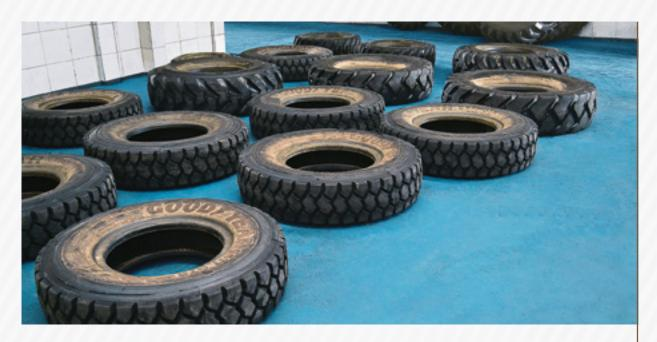
Keep the tyre/tire in the horizontal position for cooling.
