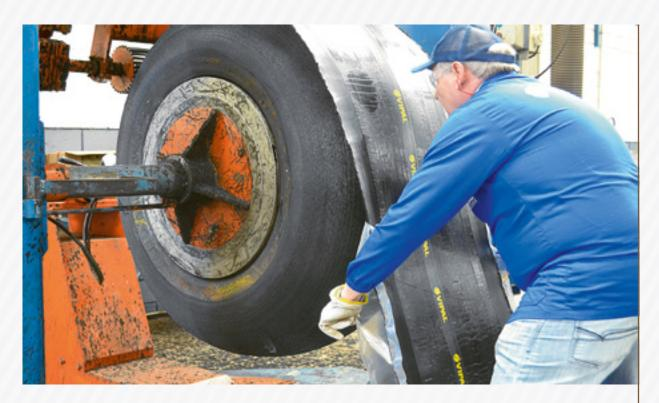
Carefully continue applying the Camelback, partially removing the plastic and ensuring that it is well centered on the tyre/tire.
