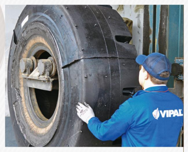
Externally, check for dislocations, failures in vulcanization and finishing.
