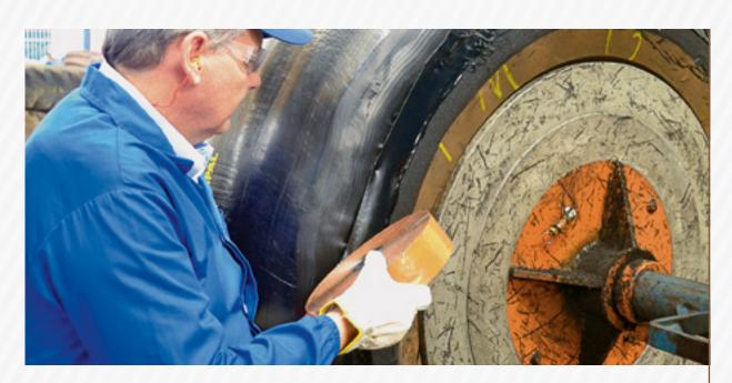
If lateral finishing is required, spread a thin layer of cement and apply tread gum or remold to the sides.
