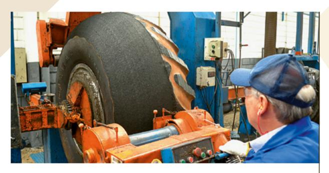
Advance carefully with each advancing so that the rubber is not burned. Excessive heating caused by great advances or older buffing blades cause superficial degradation of the rubber, which makes the adhesion of the cushion gum difficult.
