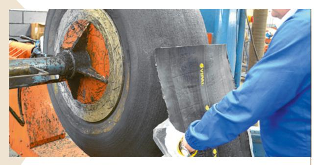
Position the tire in the machine and inflate it to 15 to 20 psi. Remove the piece of plastic from the Camelback, avoiding contact with the cushion. Center it and fix one of the tips on the tire.
