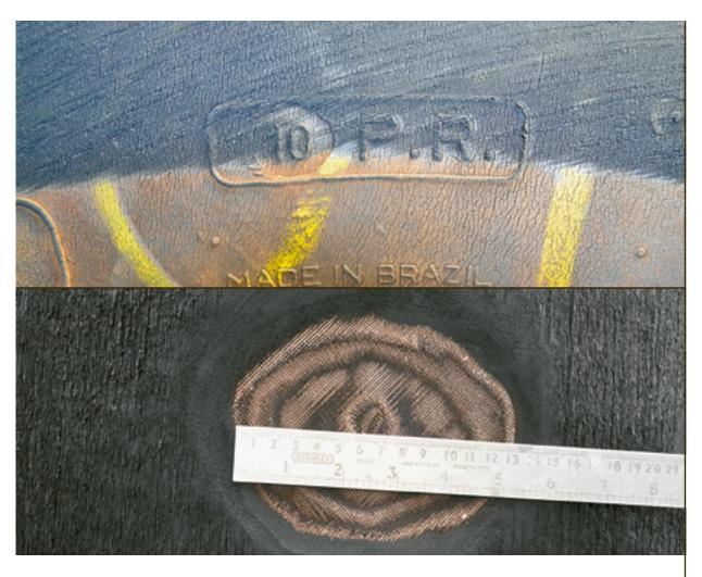
Damages should be measured on the first outer ply, disregarding the protective plies.
