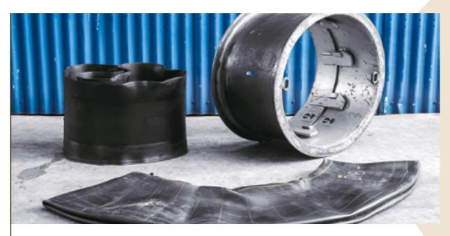
Assemble the tire with air bag, protector and wheel.
