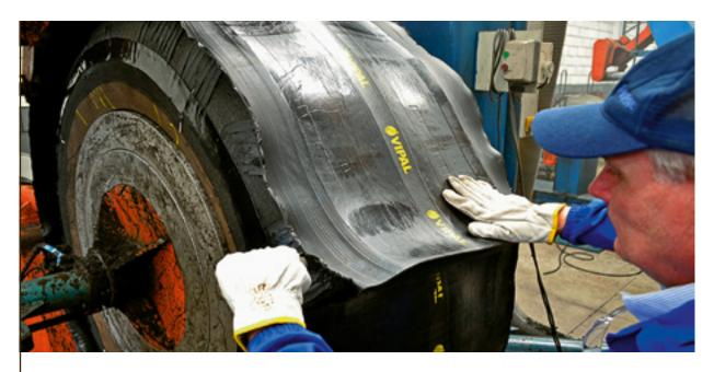
For perfect adhesion of the Camelback patch, its length should be 10 to 15 mm longer than the tire's perimeter. With the aid of a metal ruler, position the ends, hit it with a rubber hammer to increase the patch pressure, and fix it with a proper instrument.
