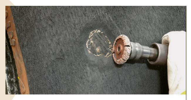
Remove the burnt rubber from the skived area with the aid of a steel brush (for tires with steel belts) or tungsten ball pin.
