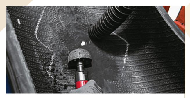
To prevent contamination and preserve the inner plies, only the demarcated area should be carefully trimmed using a fine grain carbide grinder at 2500 to 3500 rpm.
