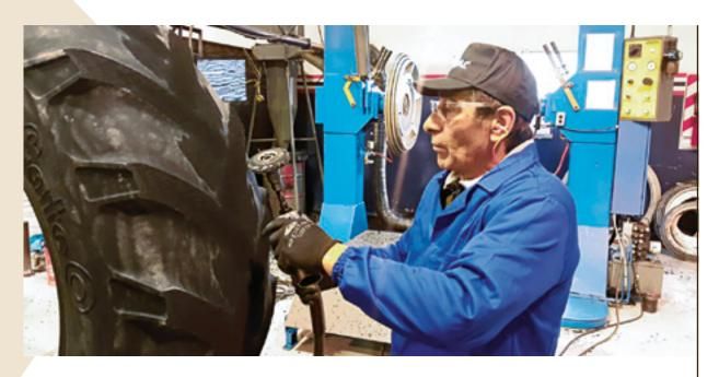
Then use appropriate material to clean between the lugs so as to enable adherence of the cover material.
