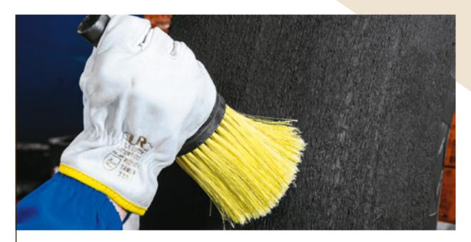
Clean the tire with a soft brush (nylon) and clean the inside with a vacuum cleaner if necessary.
