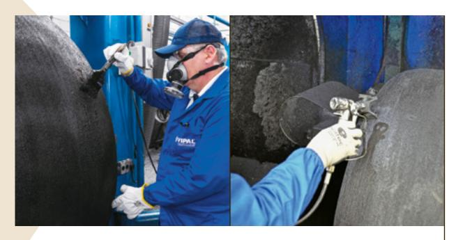
Apply a thin and even layer of cement.
