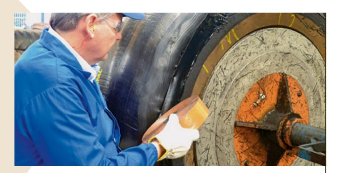
If lateral finishing is required, spread a thin layer of cement and apply laminade gum or passenger rubber on the sides.
