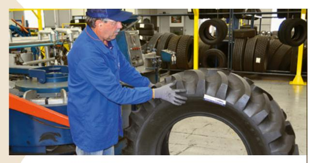
Externally, check for dislocations, failures in vulcanization and finishing.
