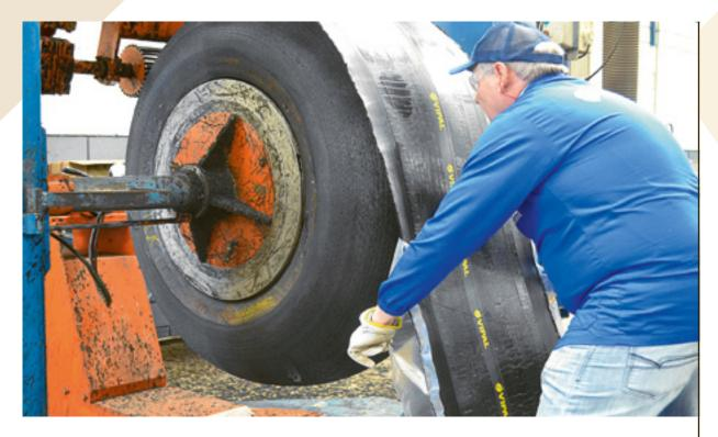
Carefully continue applying the Camelback, partially removing the plastic and ensuring that it is well centered on the tire.
