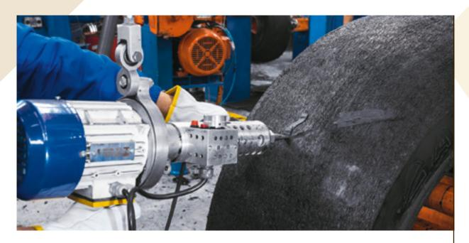
With an extruder heated to  $75^{\circ}\text{C} \pm 5^{\circ}\text{C}$ , fill the skives with Cushion gum, leaving no more than 1 to 2 mm excess above the tire level. The same is true for the sidewall.
