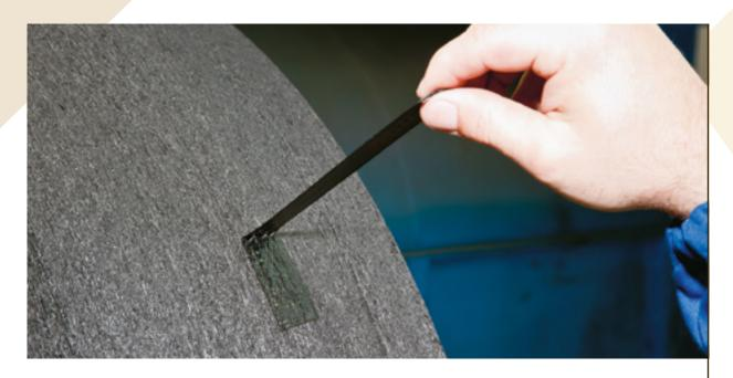
Check the complete drying of the glue before continuing the retreading process.
