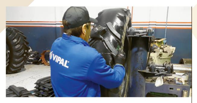
Apply the previously prepared blocks, abiding by the positioning of the original lugs.
