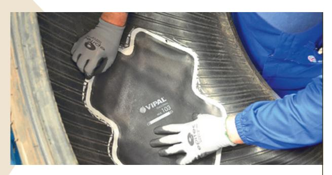
Keep the tire in normal position, without opening the beads. Position the template or patch at the center of the damage and mark the outline with chalk.
