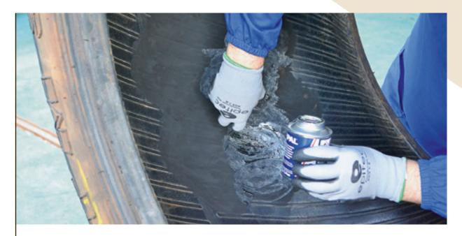
Apply vulcanizing cement to the area to be repaired, waiting for the cement to dry properly. Don't use devices for drying and avoid direct contact with the previously prepared area.
