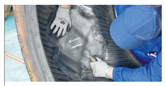
Roll the patch from the hump to the edges, ensuring better adhesion and preventing air occlusion.
