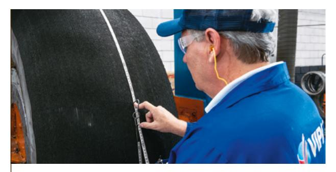
Measure the perimeter with a measuring tape, a mechanical measurer, or laser.
