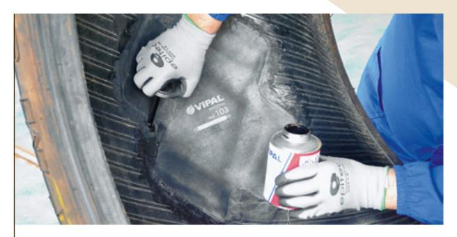
Apply sealant at the edges of the patch, covering the buffed area and protecting the patch from possible infiltration.
