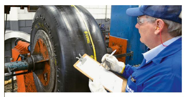
Measure the perimeter to check the measurements.
