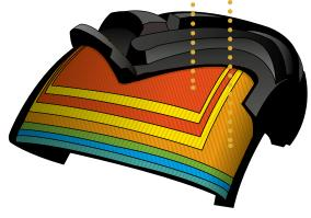
**Mixed tyre/tire construction:** a carcass with bias-ply structure and steel and nylon circumferential belts.
