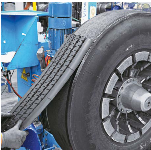
Applying tread with MB/AC cushion gum.
