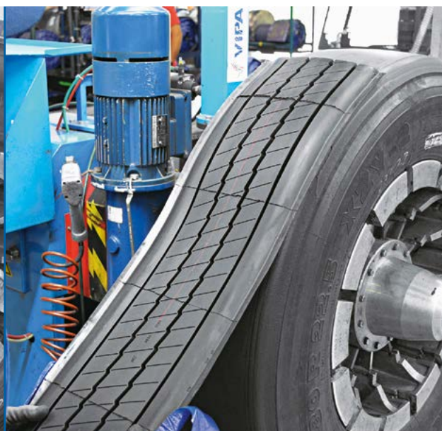
Applying tread with cushion gum to the casing (orbicushion).
